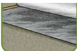
If you prefer not to work with a wooden frame, curb stones to which the artificial turf can be glued can be used as an alternative.
